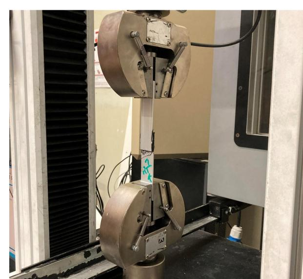
**Figure 2 –** Experimental setup for the vibrational data (Left) and Experimental setup for the tensile test of the 11 experimental samples (Right).
