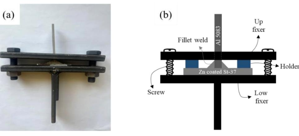
Figure 2. a) The fixture used to evaluate the strength of Teejoints. b) Schematic of the tensile testing of Tee-joints.
