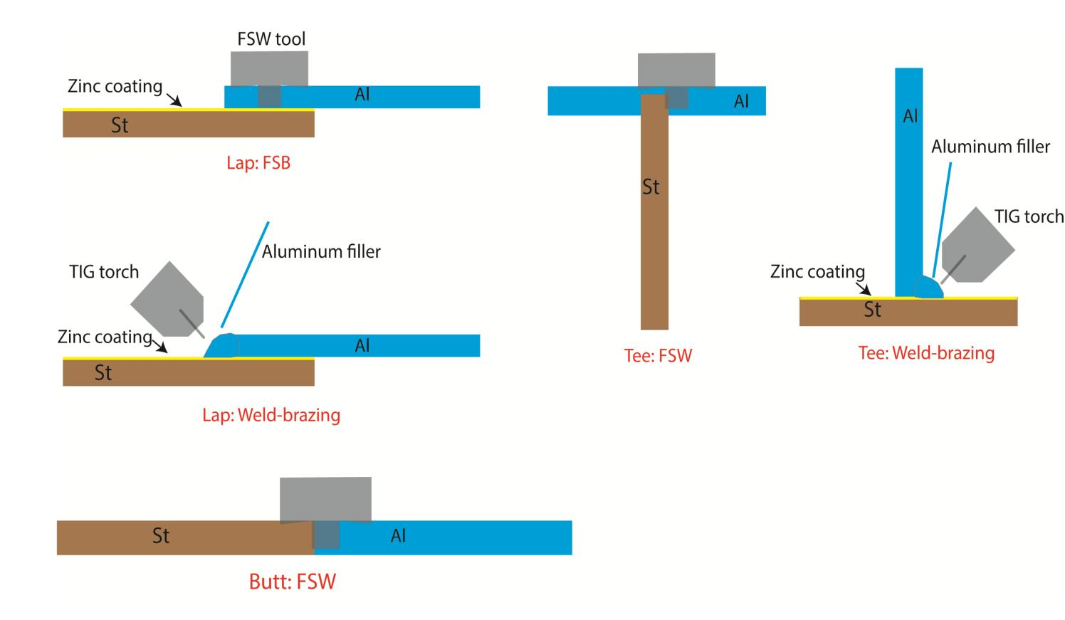
Figure 1. Various joint configurations between Aluminum and
