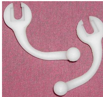
Fig. 4. Redesigned auricular pieces materialized by rapid prototyping
