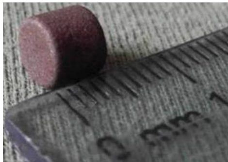
Fig. 1. Magnet used in our system for the acquisition of the 3D mandibular movement
