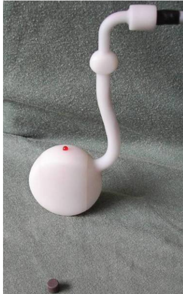
Fig. 7. Sensors support developed and the magnet used in the acquisition of the 3D mandibular movement
