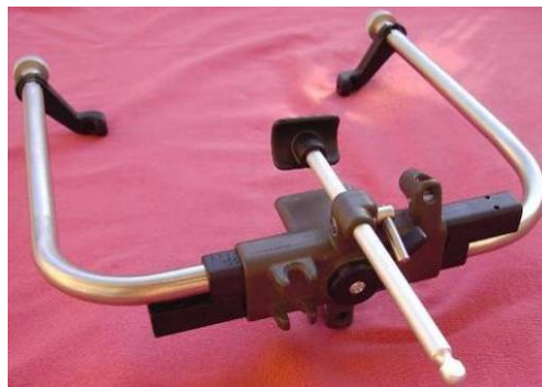
Fig. 3. Facial arc Arcus from Kavo used as the main support system of our prototype system
