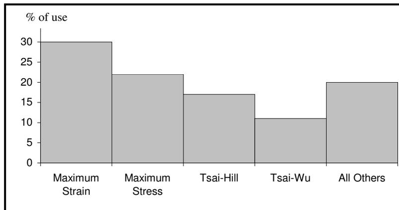
Figure 2: Industrial usage of composites failure criteria (after [11])
