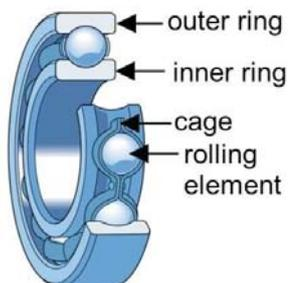
Figure 1. Main components of the rolling bearing [12].
