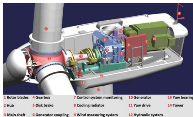
Figure 4. Structure of the studied WTs with its major components, [17].
