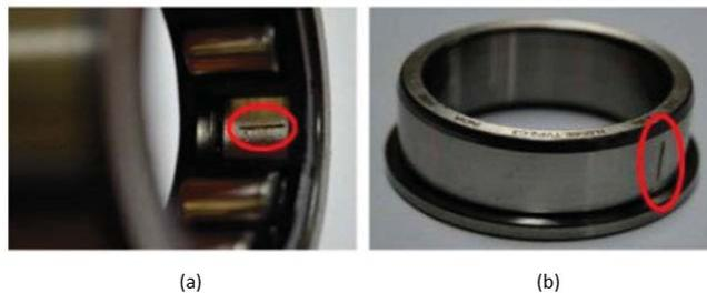
Figure 2. Bearing faults: (a) bearing crack on the inner surface; (b) bearing crack on the outer surface, [14].
