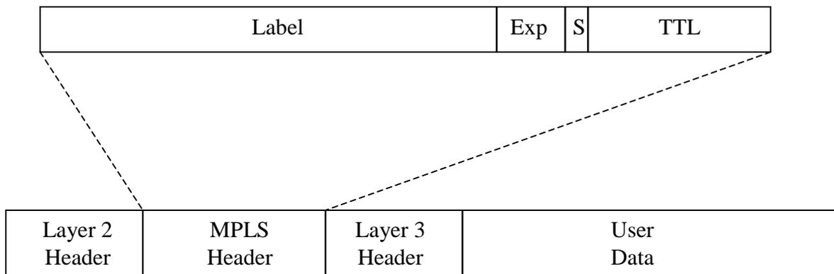
Figure 3 – MPLS header and encapsulation
