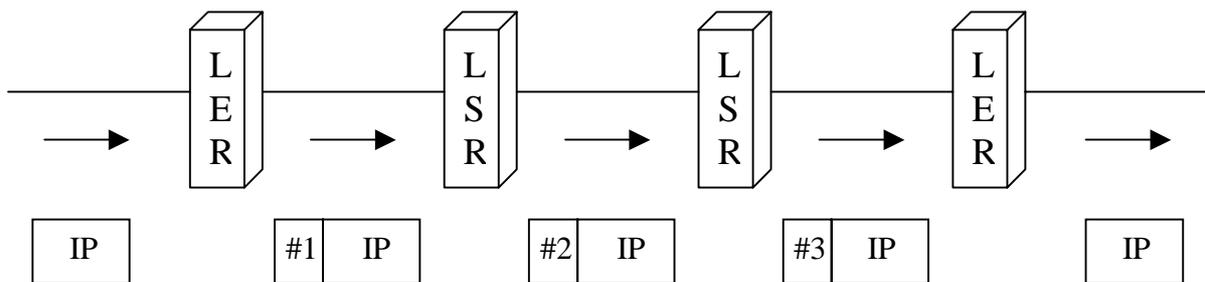
Figure 2 – Label insertion, swapping and removal
