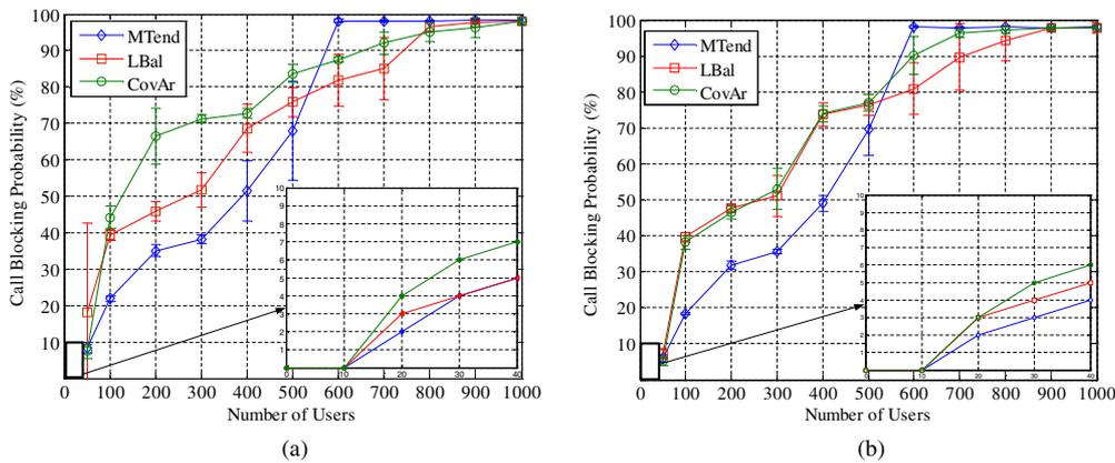
Fig. 4. Call blocking probability, without (a) and with (b) call renegotiation
