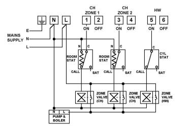
ChannelPlus H37XL Controlling 3 x two port spring return zone valves via RoomStat and CylinderStat giving independent control of Hot water and two zones of Heating
