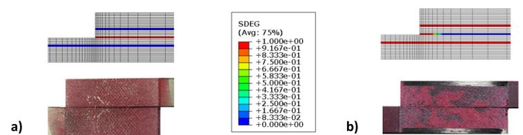
Figure 7 – Failure mechanism obtained numerically and experimentally a) CFRP+25%Al and b) CFRP+25%af under intermediate loading
