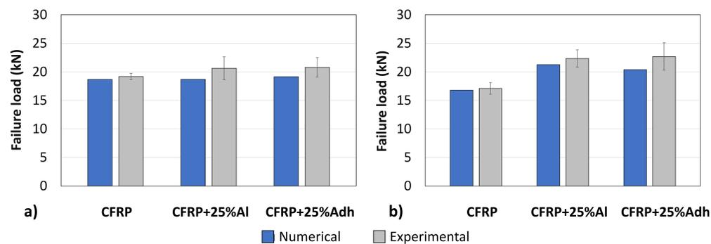
Figure 8 – Experimental and numerical failure load under a) quasi-static (1 mm/min) and b) intermediate rate loading (0.1 m/s)
