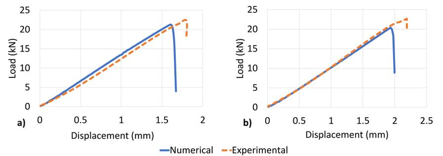
Figure 6 – Numerical and experimental load displacement curves a) CFRP+25%Al and b) CFRP+25%af under intermediate rate loading
