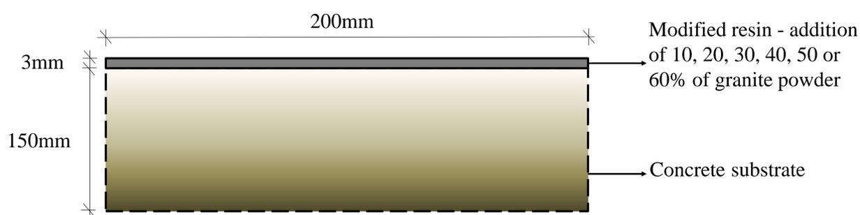
The test began with the preparation of the substrate, made of C30 / 37 concrete, S3 consistency, supplied by a specialized company. After its full hardening, the surface was ground and degreased. The resin used consisted of two components: A and B. After the first component was measured out, a measured amount of granite powder was added. After mixing, component B was added and mixed again. The modified resin was then applied to the substrate to obtain a 3mm layer.
