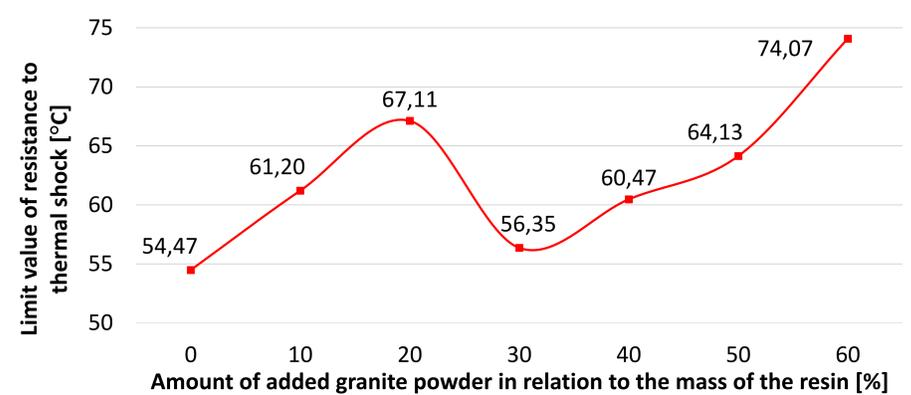
Fig. 2. Dependence of the thermal shock resistance limit on the amount of granite powder added to the resin.
