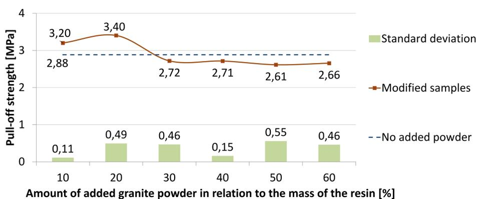
Fig. 1. The dependence of the strength on the amount of granite powder added
