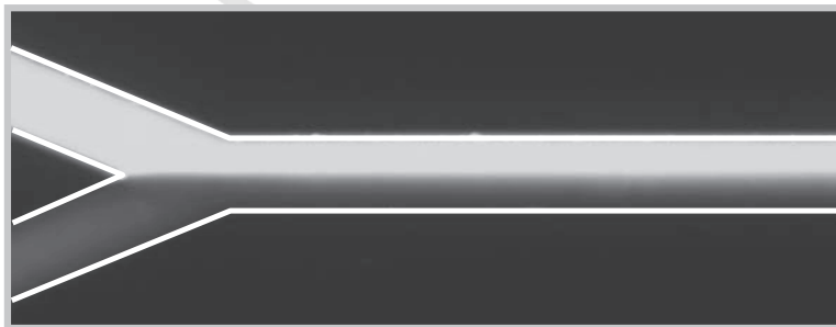
Figure 6.4 Junction of two Newtonian fluid streams in a microfluidic device under low Re flow conditions.
