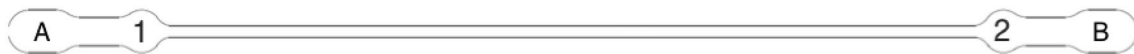
Fig. 2 Schematic of the straight microchannels with two pressure holes (1 and 2), and one entrance (A) and exit (B) ports
