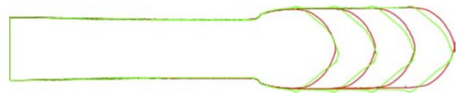
Fig. 6. Numerical simulation of extrudate swell with Re = 0.5 and Wi = 0.3 using the log-conformation tensor (red curve) and the extra-stress tensor (green curve). Visualisation of the free surfaces at dimensionless times t = t^* \frac{U}{R} = 12.5, 15, 17.5, 20 .
