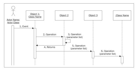
The internal workings of Object 1 that led to the creation of the message, and the internal workings of Object 2 that led to the return message, are not shown in sequence diagrams. (Details of the inner workings of the objects are represented in another type of diagram called an activity diagram - which we'll see in the next phase of the UML design process.)
