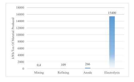
Fig. 3. Electricity consumption of aluminium production processes [28].
