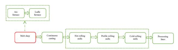
Fig. 4. The steel industry supply chain.
