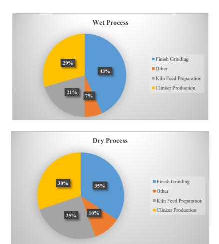
Fig. 6. Energy consumption of typical wet and dry cement plants based on processes.
