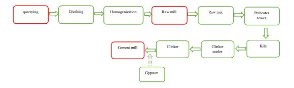
Fig. 5. -Supply chain of a typical cement plant.
