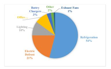
Fig. 7. Energy consumption of a typical refrigerated warehouse.
