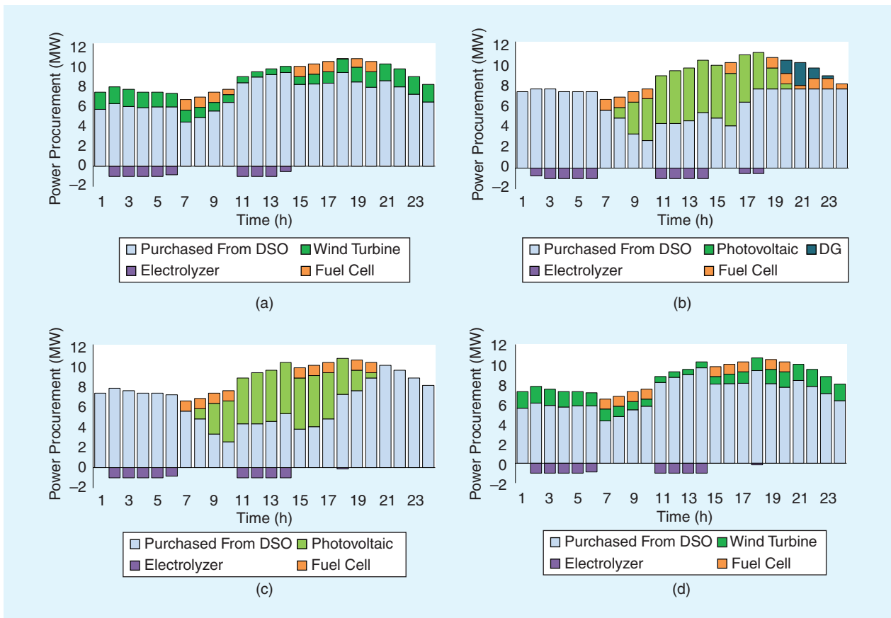
FIGURE 10. Power dispatch in the microgrids. MG: microgrid. (a) MG1, (b) MG2, (c) MG3, and (d) MG4.
