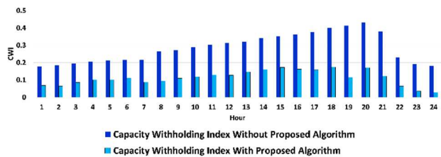
Fig. 17. The CWI values for scheduling horizon with and without the proposed algorithm.
