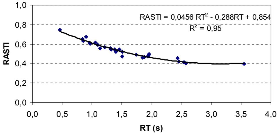
**Figure 7:** Example of a regression model for the relationship between the *RASTI* and the *RT* room averaged values (500/1k Hz).
