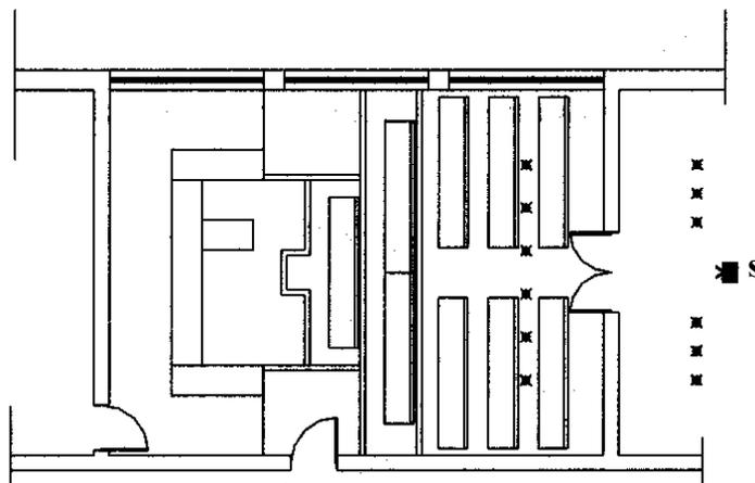
**Figure 6** - Standard location of the twelve measuring points and sound source ( $S$ ) for the  $D_{n,w}$  airborne sound insulation measurements.
