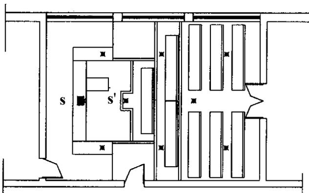
**Figure 5** - Standard location of the eight measuring points and sound source ( $S$ ) for the  $RT$ ,  $EDT$ ,  $TS$ ,  $D_{50}$ , and  $C_{80}$  measurements. For *RASTI* measurements the sound source was also put in the  $S'$  position (facing  $S$ ): two sets of measurements.
