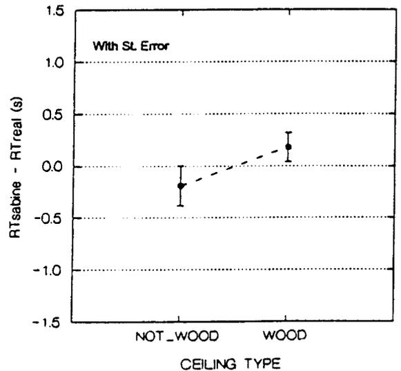
Fig. 4 - Analysis of the effect of ceiling type (*wood* and *non wood*) differences ( $RT_{REAL} - RT_{SABINE}$ ). Mean values for all the churches in each ceiling type are shown with one stand. error confidence interval.
