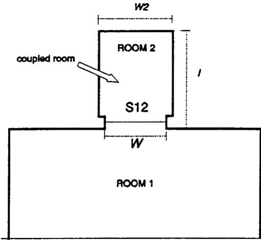
Fig. 1 - Plan sketch of a general church with a coupled space. *l*-length, *S*<sub>12</sub>-opening surface area, *w*-opening width, *w*<sub>2</sub>-coupled space width, Room 1-main room, Room 2-coupled room.
