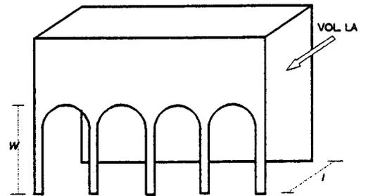
Fig. 2 - 3-D sketch of lateral aisles in a general church. *l*-width of lateral aisle, *w*-width of opening to lateral aisle, vol<sub>LA</sub>-volume of lateral aisle.
