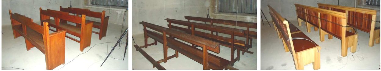
Fig. 1 (left), 2 (center) and 3 (right) – Pews type F (left), type A (center) and type N (right) in the reverberant chamber. 3
