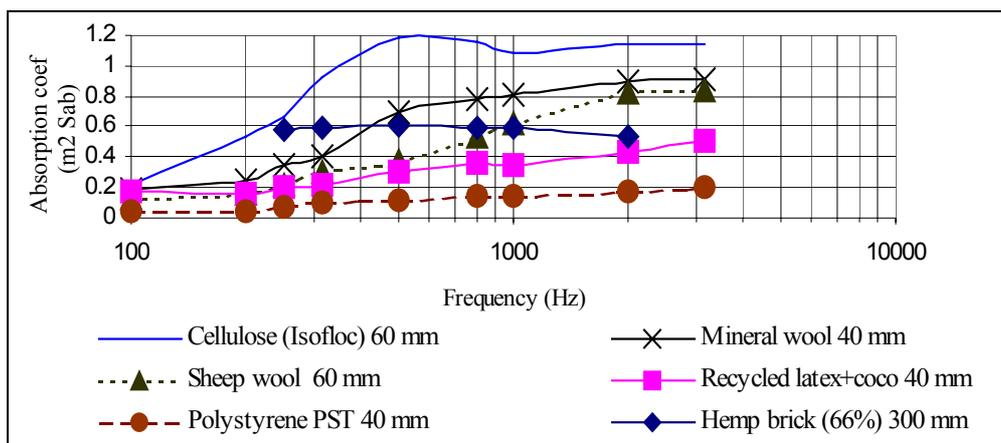
Figure 3 – Sound absorption coefficient of various materials
