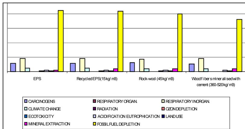
Figure 2 - Evaluation (in points) for insulation layers by the Eco-indicator '99.
