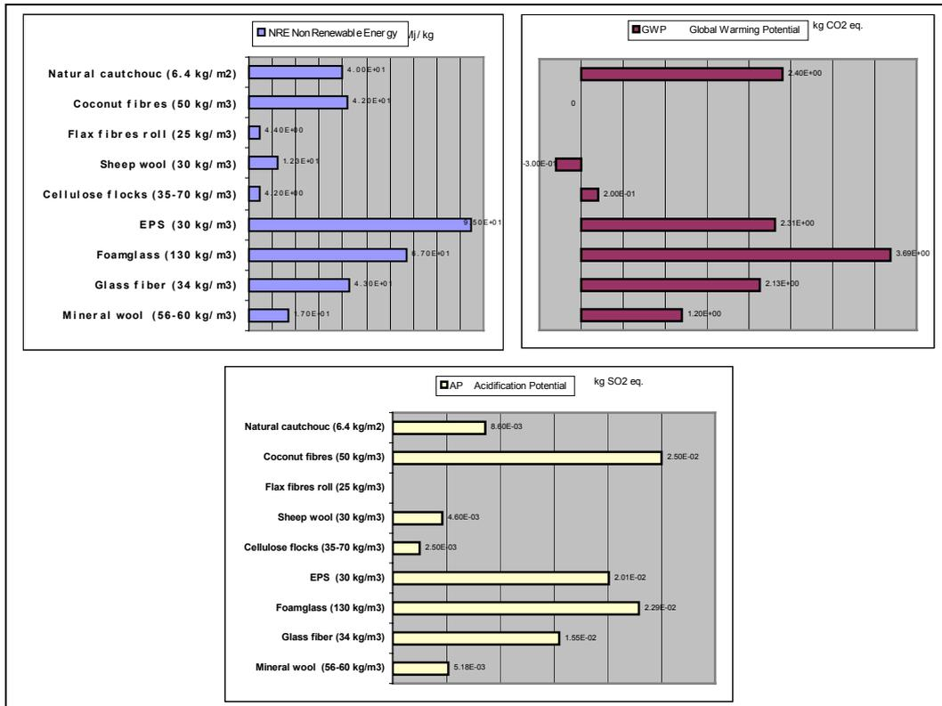
Figure 1 – Comparison of environmental impacts of traditional and natural insulations from cradle to gate. Sources: Ecoinvent, ETH-ESU (CH), IBO (A)
