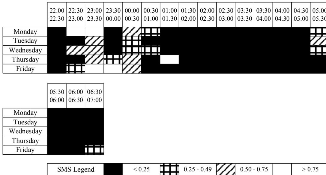
Figure 7. SMS variation in four groups of values within pre-defined time intervals - nighttime period (allowable error of  $\pm 1.0$  dB(A))
