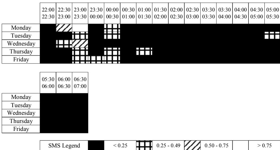
Figure 6. SMS variation in four groups of values within pre-defined time intervals - nighttime period (allowable error  $\pm 0.5$  dB(A))
