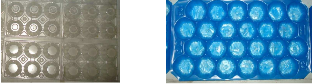
Fig. 12 and 13 – (left) BP12 - Boxes of plastic for 12 eggs when the inverse surface is facing up; (right) TPF24 - Trays of plastic for fruit with 24 cavities when the normal surface is facing up.
