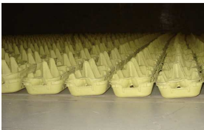
Fig. 8 and 9 – (left) B12A-o-n-WL – Boxes (open) for 12 eggs (with small apertures) without lids with the normal surface facing up (normal surface about the lids); (right) B12-o – Boxes (open) for 12 eggs when the inverse surface is facing up.
