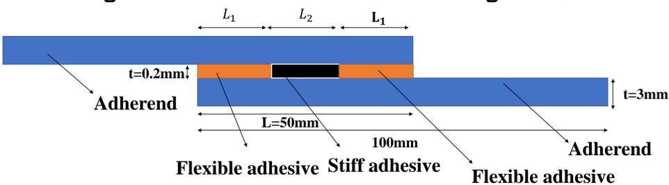
Figure 2 - SLJ specimen geometry (SLJ width= 20 mm)
