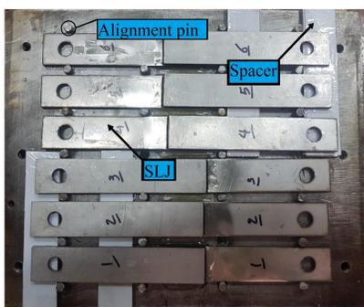
Figure 1 - Mold used for the manufacturing of SLJs
