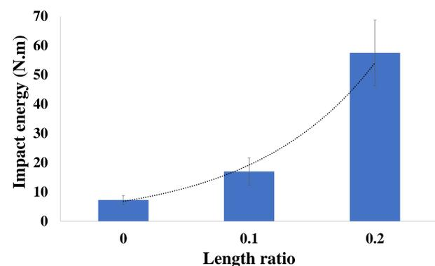
Figure 5 - Fracture energy of the adhesive at impact
