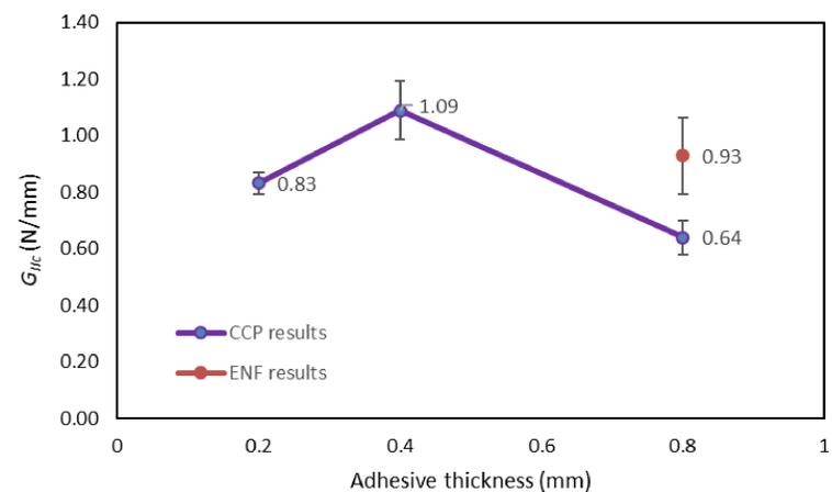
Figure 5 – Shear fracture energy, Effect of specimen type and adhesive thickness
