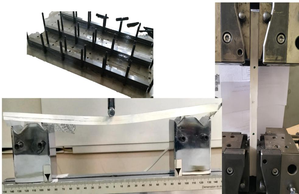
Figure 2 – CCP and ENF specimens (manufacturing and testing)
