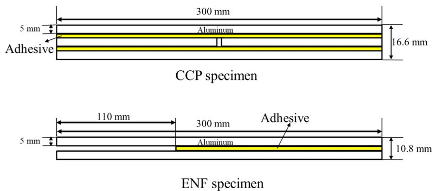
Figure 1 – Geometry of the tested joints.
