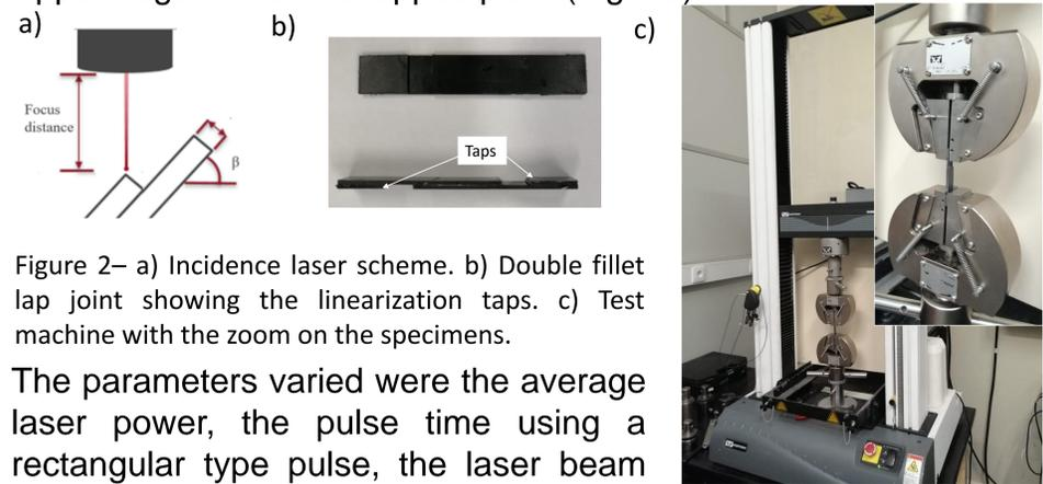
Figure 2– a) Incidence laser scheme. b) Double fillet lap joint showing the linearization taps. c) Test machine with the zoom on the specimens.
