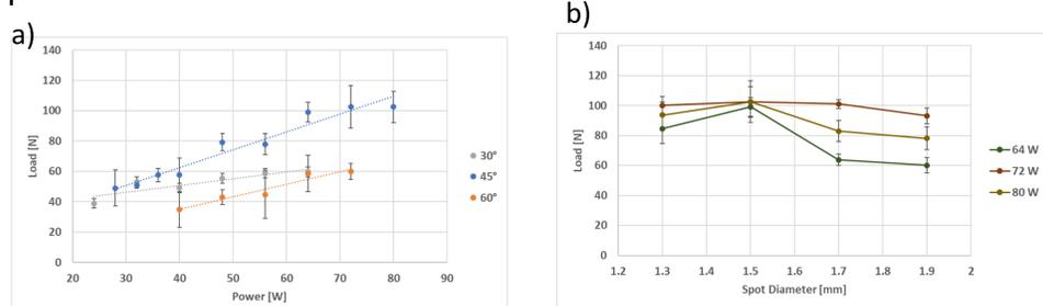
Figure 3 – a) Results of the failure load in relation to the angle of incidence and average power. b) Failure load study for 45° angles, with pulse time fixed in 1.5 ms varying the average power and the laser beam diameter.
