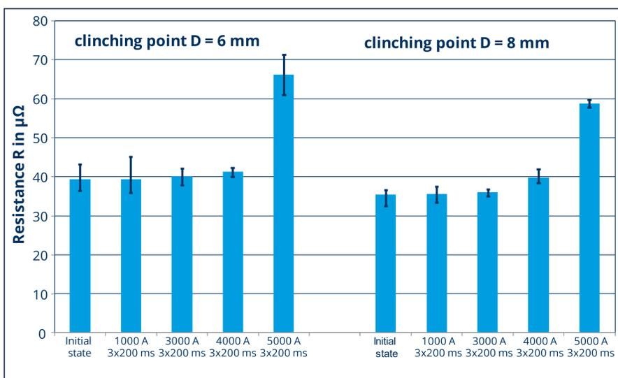
Within the framework of preliminary tests, clinched joints with a point diameter of  $D = 6$  mm and  $D = 8$  mm were examined. It can be seen that the resistance does not increase at all or only increases slightly up to a current of 4 kA. When the samples are loaded with a short-circuit current of 5 kA, a significant increase in the connection resistance can be seen. The increase in resistance is greater at the clinch point with a size of  $D = 6$  mm due to the smaller contact area.
