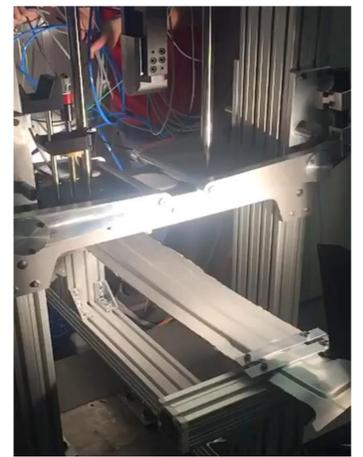
Figure 8 – Testing procedure for impact testing of full-scale bonded joints.
