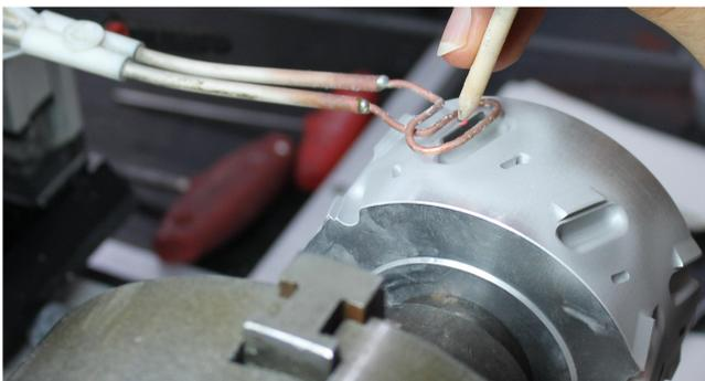
Figure 1 – Induction cured prototype manufacturing.
