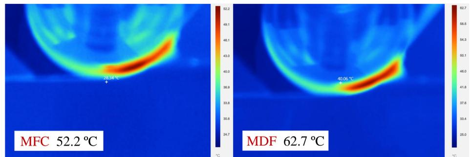
Figure 3 – Thermal imagery of different woodworking scenarios, MFC (melamine faced chipboard) and MFD (medium density fiberboard).
