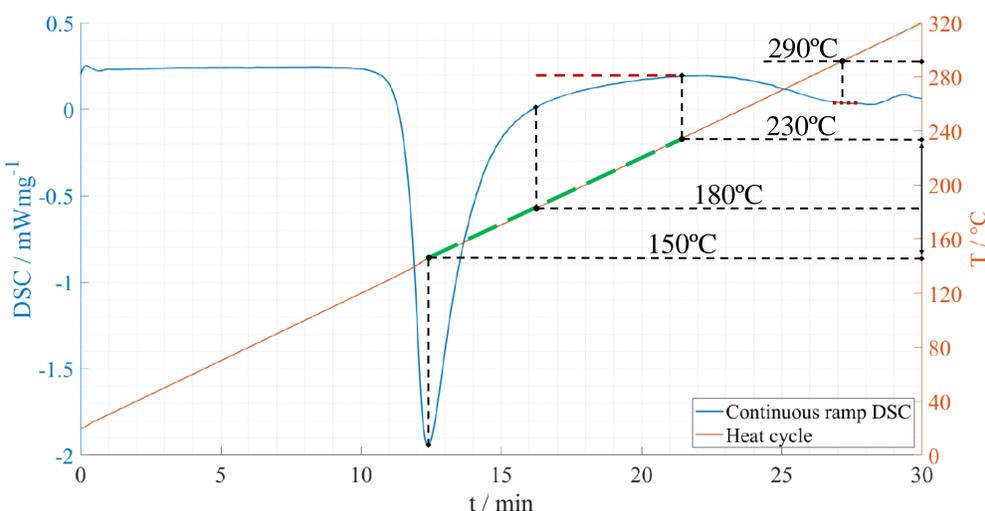
Figure 2 – DSC curves for the continuous ramp heating cycle.
