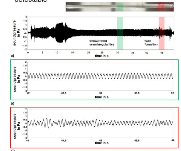
Figure 7: a) FSW weld seam and sound pressure b) without weld seam irregularities, and c) during flash formation
