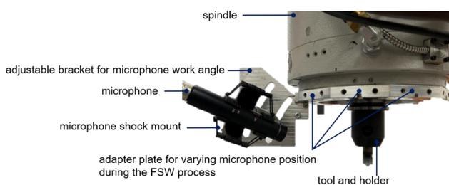
Figure 2: Measurement setup for the recording of the emitted airborne sound
