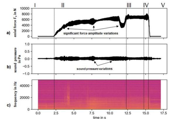
Figure 5: a) Axial force  $F_z$ , b) sound pressure, and c) spectrogram of the acoustic signal as a function of time and process stages I-V
