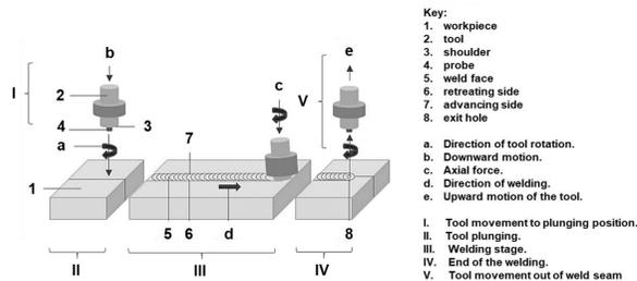
Figure 1 : FSW operation principle and process stages
