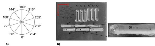
Figure 3: a) varying rotation angles compared to the welding direction and b) FSW weld seams joined in  $\pm x$  and  $\pm y$  direction with an enlarged section of a weld seam
