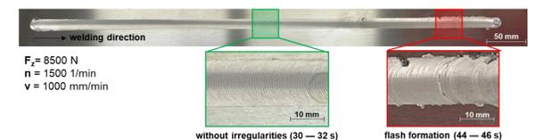
Figure 6: Varying surface quality at the center and end of the weld seam
