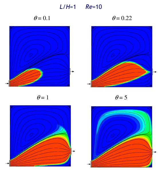
These pictures clearly illustrate that approximately at  $\theta$  = 0.22 one starts to 'see' tracer at the reservoir outlet. In addition, even for a very long time of operation (about 5 times the residence time), the reservoir is not completely full of tracer, due to the large stagnant zone.
