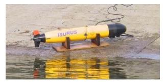
Fig. 2. The *Isurus AUV*. IV. IN-SITU MEASUREMENTS
