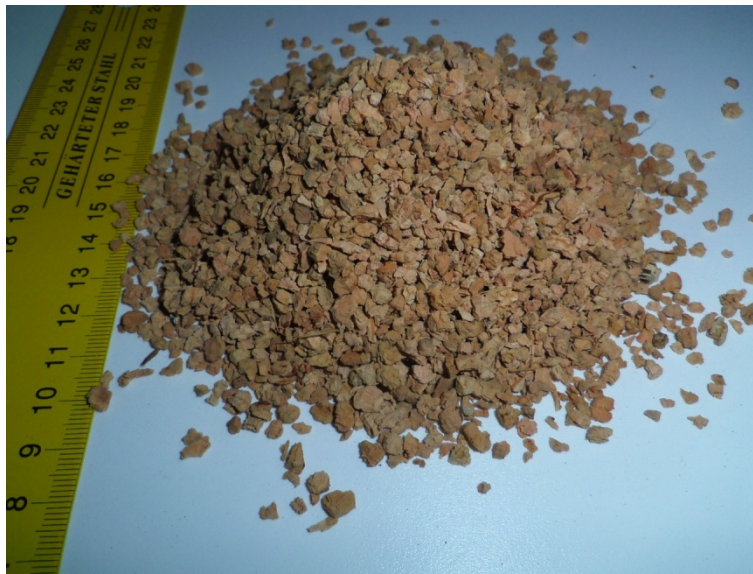
Fig. 2. Granulated cork having a particle size exceeding 5 mm and a density of 90 kg/m 3 .
