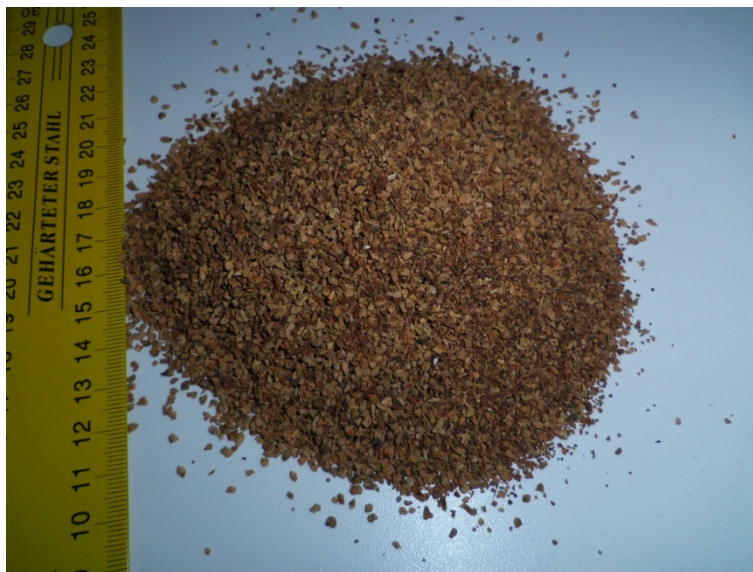
Fig. 3. Granulated cork having a particle size greater than 2 mm and a density of 120 kg/m 3 .
