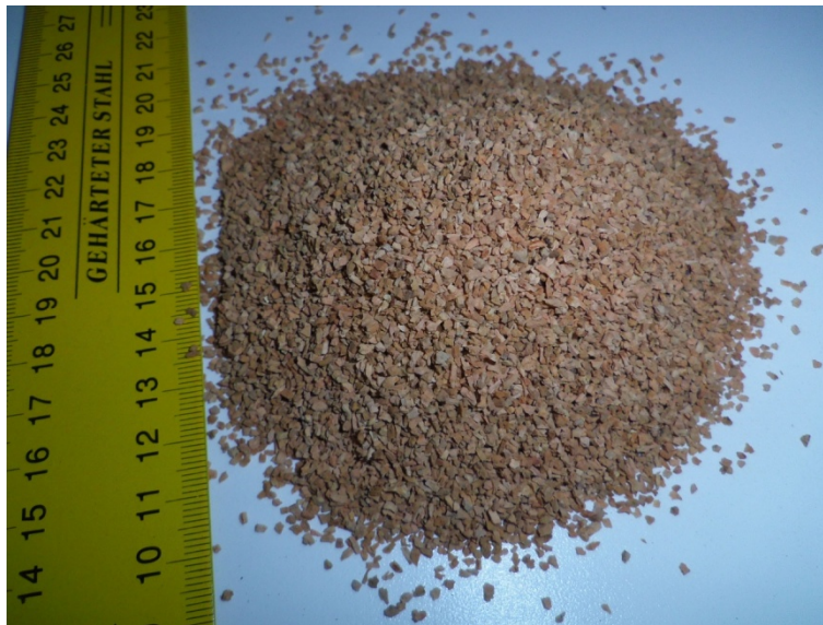
Fig. 4. Cork dust having a particle size smaller than 2 mm and a density of 60 \text{ kg/m}^3 .
