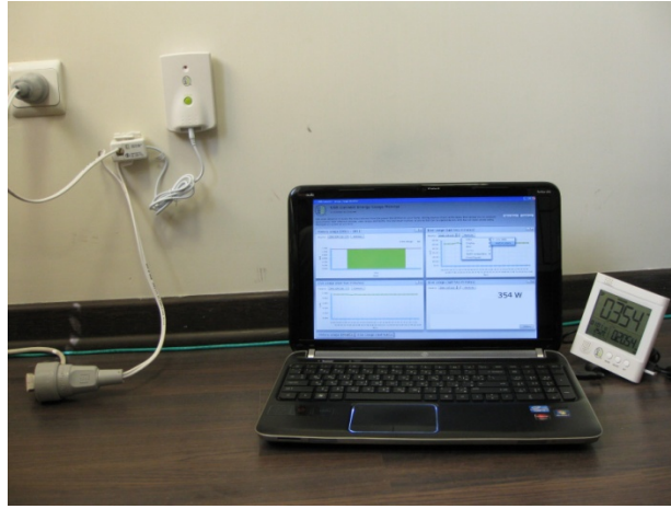
Fig. 5. The laptop power consumption measurement
