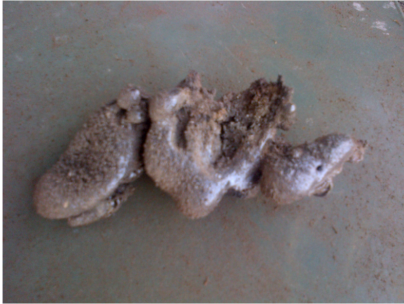
Fig. 3. Vitrified ash collected in a thermal oil boiler fuelled with woodchips.
