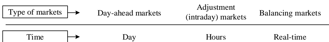
Fig. 6: Different time scales of operation problem regarding the clearing time of the markets
