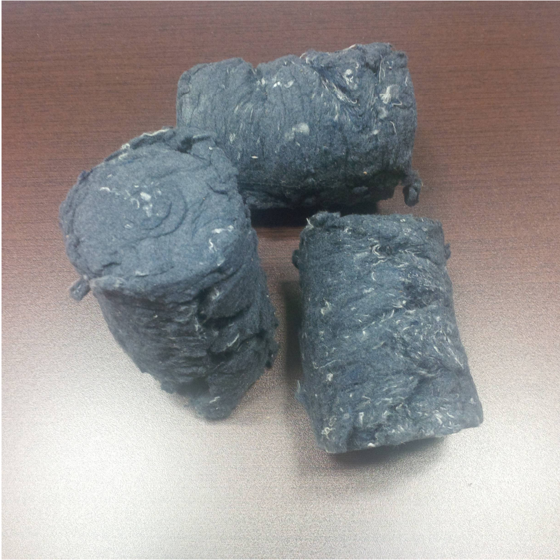
Figure 5. Briquettes composed of a mixture of cotton (90%) and polyester (10%).
