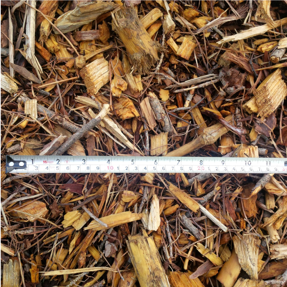
Figure 3 – Common visual aspect of the Pinus pinaster woodchips used in this study.
