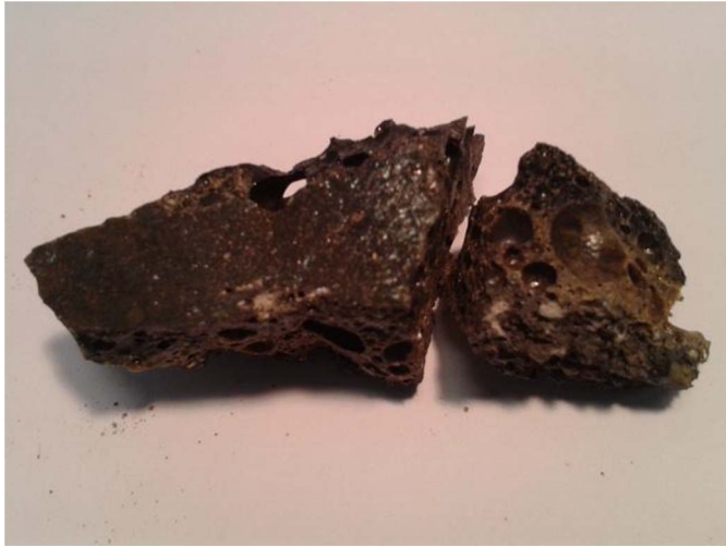
Fig. 1. Vitrified sample of ash collected in an industrial boiler.
