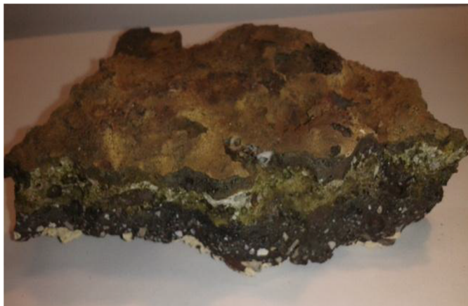
Fig. 2. Sample of “petrified” ash collected in an industrial boiler. It is possible to identify several layers with different chemical compositions.
