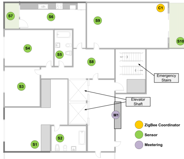
Fig. 16. Home configuration with the position of the ZigBee coordinator, sensor and metering.
