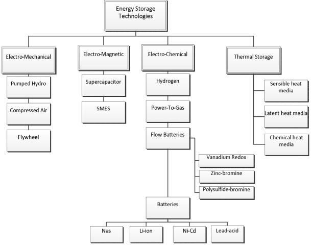
Fig. 5. The main classification of energy storage systems [22]
