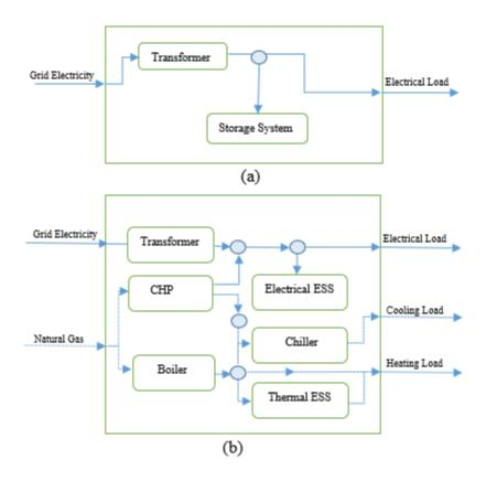
Fig. 8. Multi-energy structure in presence of ESS [42]
