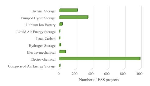
Fig 4. The various ESS technologies [8]
