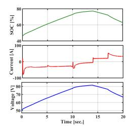
Fig. 6. Voltage, current and SOC changes of supercapacitor
