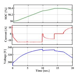
Fig. 5. Voltage, current, and SOC changes of battery
